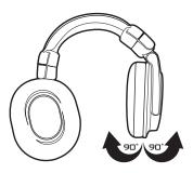
Rotatable earcup for comfortable single-ear monitoring as shown in the illustration. Rotating earcup stops in place.
