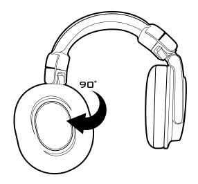
Rotatable earcup for comfortable single-ear monitoring as shown in the illustration. Rotating earcup stops in place.
